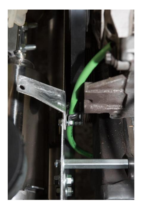
6. Slide the black plastic routing clamp over the dipstick tube so that the bolt hole on the clamp lines up with the bolt hole on the right side of the bracket. Insert a bolt through the clamp and bracket and loosely install a nut onto the exposed threads.
