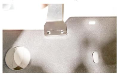
Mark the heat shield through the left hole and remove the bracket. Center punch at your mark and carefully drill a new hole with a 1/8" and then a  $\frac{1}{4}$ " bit. Use a file to slot the new hole to match the existing hole.
