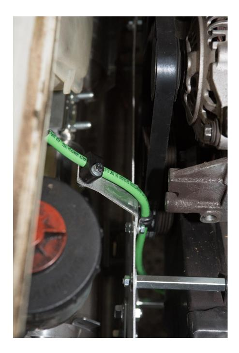
7. Position the tube so that it runs in as vertically straight as possible. Be very aware of the crankshaft pulley and ensure that the dipstick tube clears the pulley with plenty of space. Tighten the fasteners making sure that the dipstick doesn't shift while doing so.
