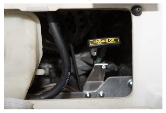
9.Prime and install Subaru filter and fill with approximately 4.5 quarts of 5/30 motor oil for the 2.5 liter and 10/30 for the 2.2 liter. Refer to Subaru specifications pertaining to your specific engine for oil type, weight and service intervals.
